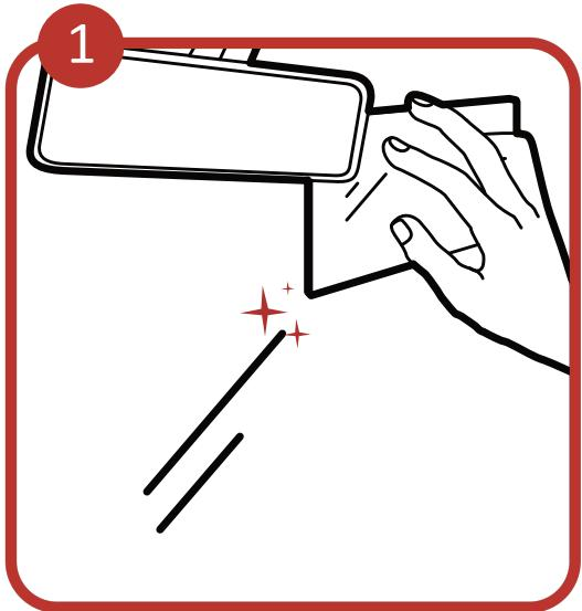
Clean the windshield and paste the electrostatic film onto it.
