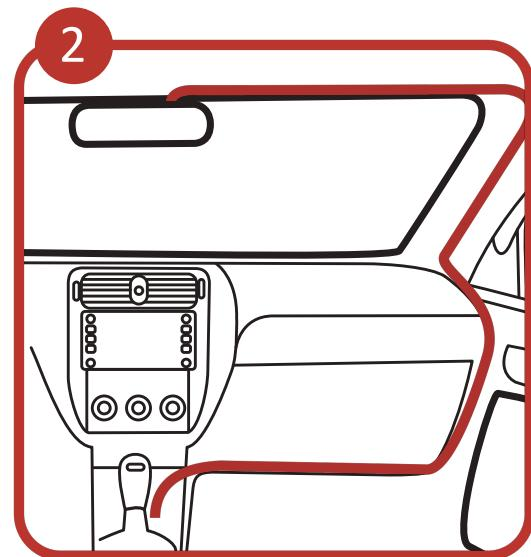
Paste the device onto the electrostatic film and route cable to the disaster box for power supply.
